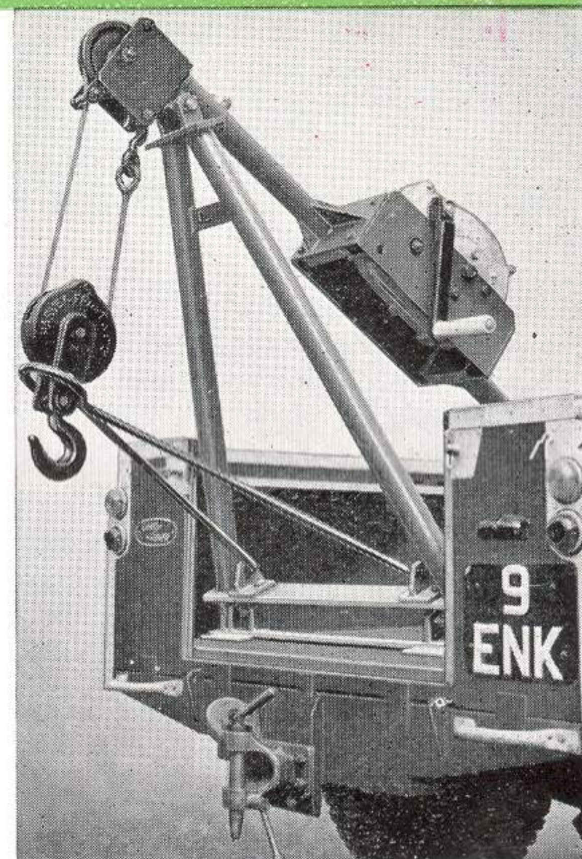
Crane mounted on Land Rover showing Anti-Sway Bar in position.
