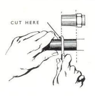
Slit cover and peel off cleanly down to wire braiding.
