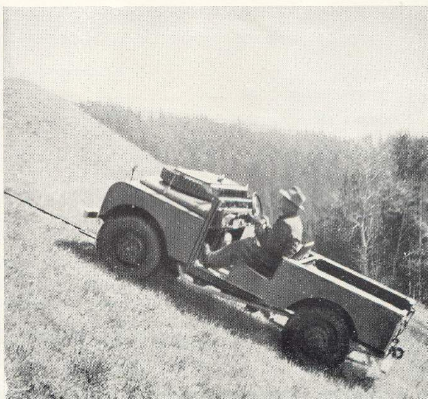
LAND-ROVER HOISTING ITSELF WITH THE WINCH CABLE
