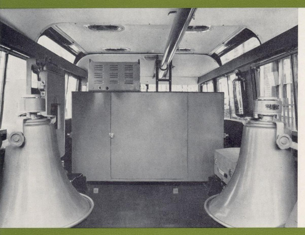
Electrical power for operation of the equipment is provided by an alternator driven by the vehicle engine.
