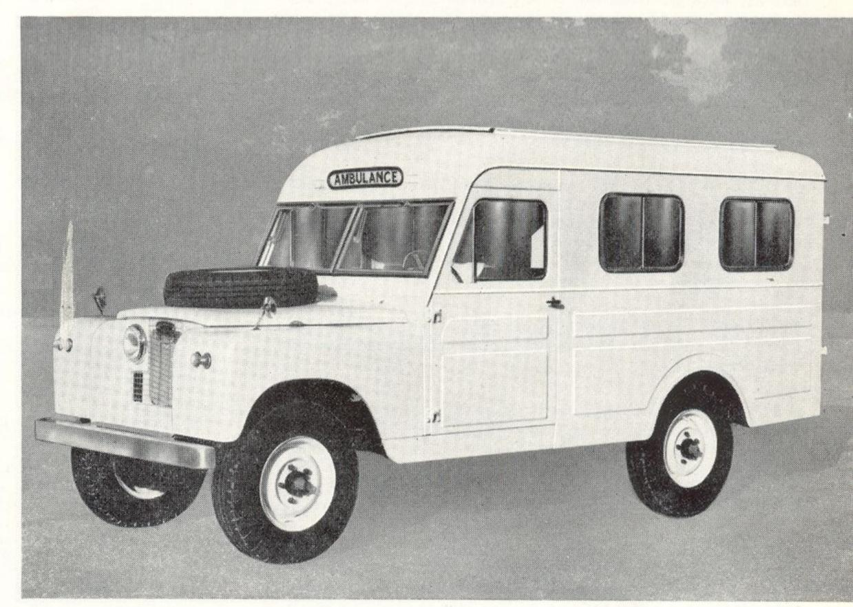
THIS up-to-date ambulance incorporates the latest aluminium alloy construction techniques to combine toughness with comfort, and has all the mobility and tenacity afforded by a four-wheel drive.
